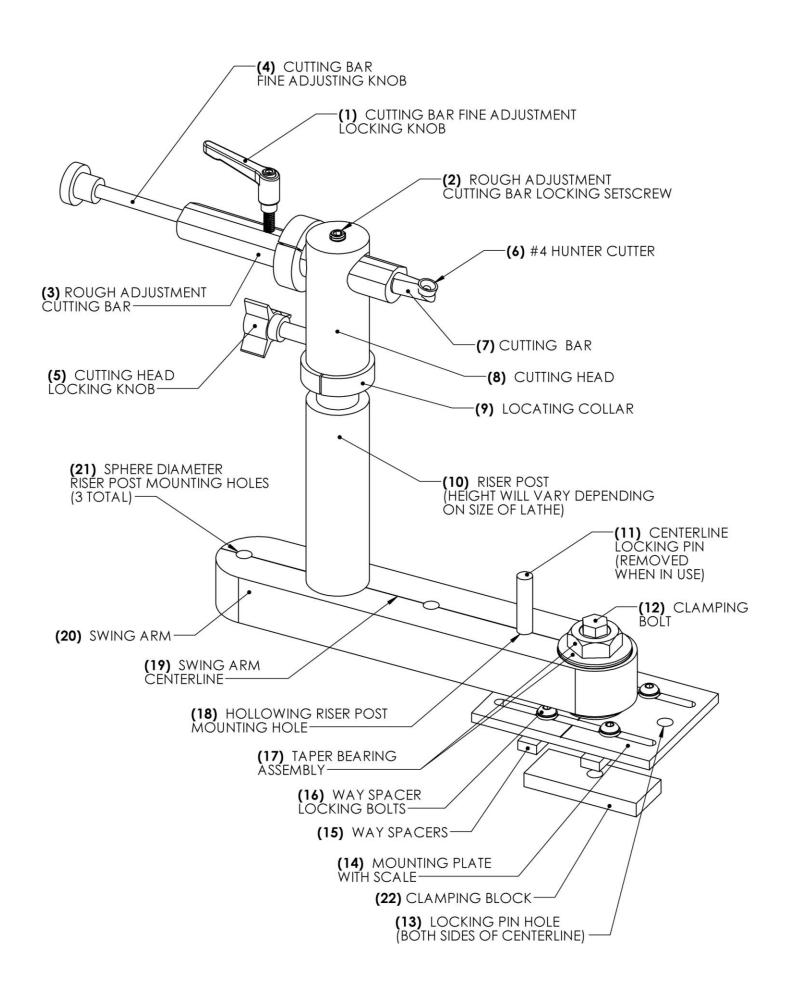
1. Loosen Cutting Bar Fine Adjustment Knob (1) and Rough Adjustment Setscrew (2). Insert Cutting Bar (7) into Rough Adjustment Cutting Bar (3) with flat of Cutting Bar (7) facing up. Lightly tighten Cutting Bar Fine Adjustment Knob (1) on flat of Cutting Bar (7).
